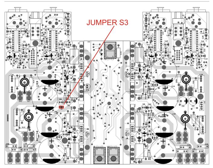
Switching to high speed fan mode is made by inserting a jumper connection inside the amplifier. High speed fan mode (fan is controlled by signal input) may be desired with ultra high and critical operational condition. Please find the location of this jumper S3 in the diagram above. Please note that we recommend the jumper removal by a qualified technician.
